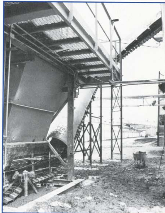
THE SERPENTIX CONVEYOR AT Stony Point is located at ground level on the corner of the waste processing building. The conveyor is seen here making its helical turn to the right and entering the building after elevating gypsum from the sizing hopper at its left.
