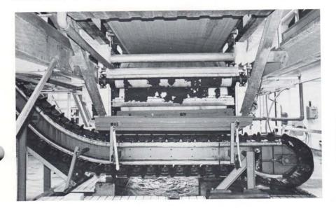
DEWATERED SLUDGE IS loaded from the filter press onto the Serpentix. The continuous path conveyor then makes a sharp vertical turn in the left of the photo to start the 45 degree climb shown in upper right photo.
