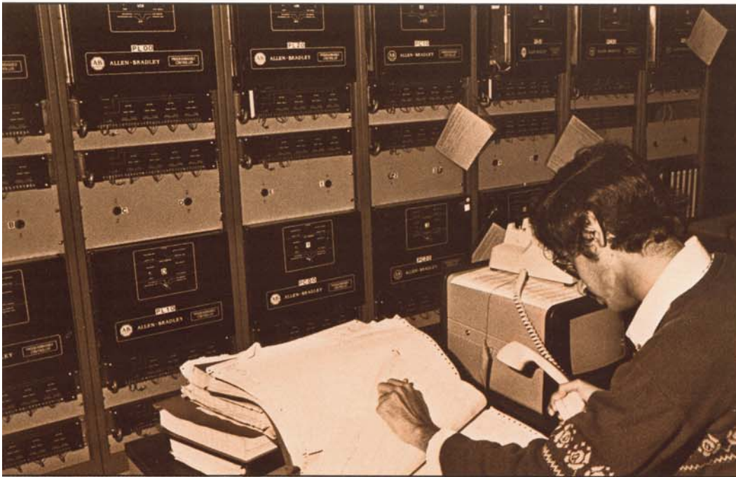
LONE STAR'S COMPUTER CONTROL Center monitors each phase of manufacturing to assure high quality control standards. A Lone Star technician double checks shell tip bore specifications and relays the information to an on-line checkpoint.
