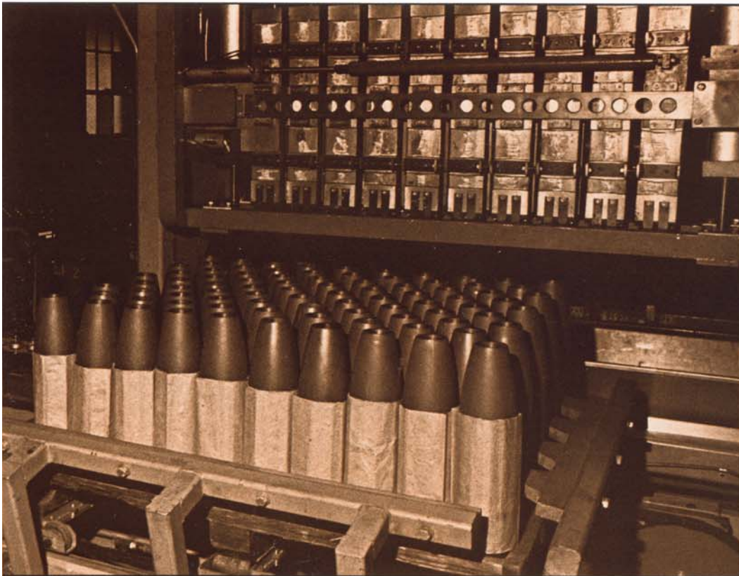
THE FIRST MANUFACTURING STAGE for incoming 105mm artillery shells at Lone Star is this depalletizing station. Once protective cardboard liners are removed, the shells are regrouped into pallets of 16 and sent along conveyor tracks to the loading stations.
