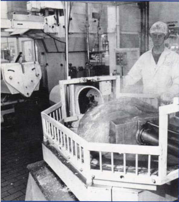
SUCRETS LOZENGES BEGIN IN THE Beecham kitchen as a large mass of taffy-like candy. After kneading by the machine in right foreground of photo above, the candy is transferred to the machine in left of photo. Soft lozenges are made by it from the candy mass and are fed onto cooling mesh conveyors in the adjoining (cooling) room.
