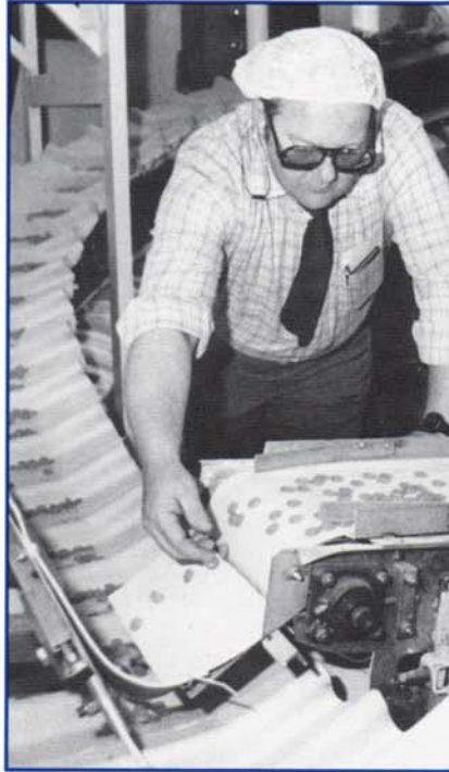
BEECHAM PLANT ENGINEER WALTER Van Dine checks lozenges at left as they are fed from the slider belt transfer conveyor onto the Serpentix Continuous Path Conveyor.
