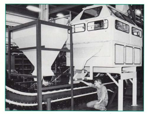
SAMPLES OF CRUSHED, UNCLEANED coal are fed onto the conveyor via the large hopper. Under the separator, a technician inspects the diverter shield and the larger outlet leading from the separator to the shield. Coal samples are fed through the separator continuously until testing of each sample is completed.
