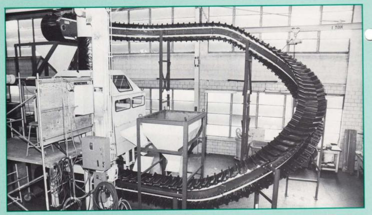
A 360 DEGREE SPIRAL by the Serpentix conveyor (above) provides a true closed loop for testing the pre-combustion coal cleaning dry separator developed by
