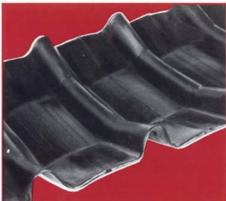
NATURAL CRADLES (PANS) are formed between the convolutions and 20-degree angles imparted to each side of the belt by stiffeners.
